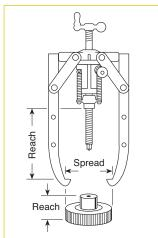
Remove gears, bearings, and other press-fitted parts with speed and ease.
