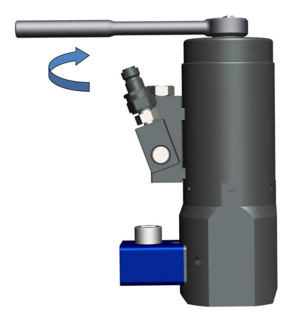
Once the Tensioner is in situ, it should still be possible to rotate the bridge to a suitable angle to access the bolt if required.
