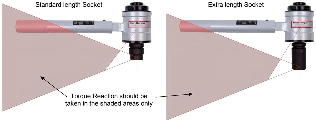
**FIGURE 5 – HT 4 Series Safe Reaction Window**
