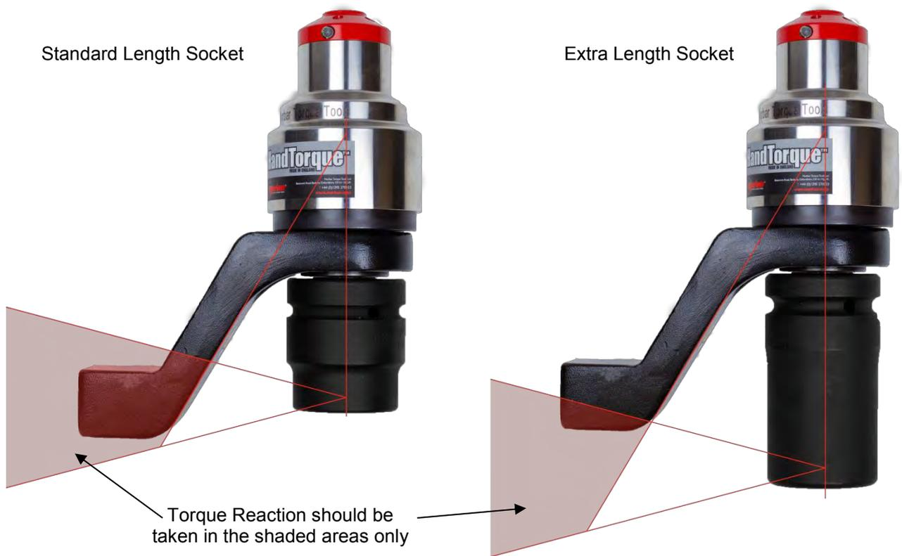
**FIGURE 6 – Compact Series Safe Reaction Window**
