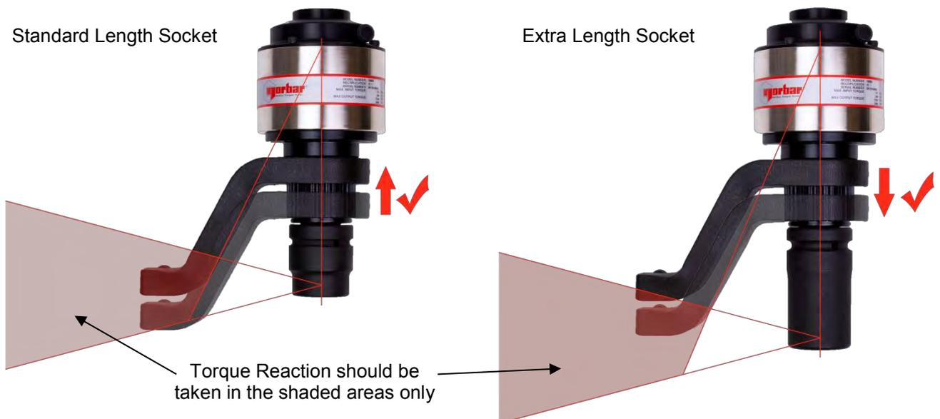
**FIGURE 4 – Small Diameter Series Safe Reaction Window**
