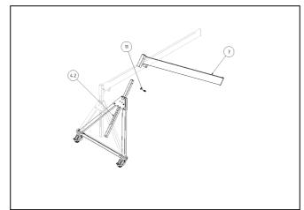
Make sure that the brakes of the wheels are fixed. Now one Person must lift the lateral stand with the long beam sleeve (4.2) and hold it as the second person plugs the beam housing (alu-square-special-profile), which is welded onto one end of the alu-beam, onto the beam sleeve.
