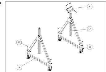
First put the horizontal adjuster (6) onto the shorter beam sleeve (4.1). The horizontal adjuster must be open.
