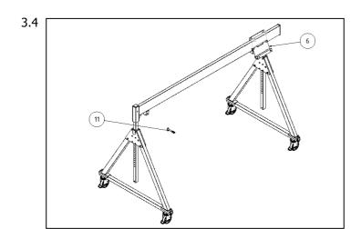
Now the second person brings the second lateral stand in an upright position so the alu-beam can be insert into the lower part of the horizontal adjuster (6).
