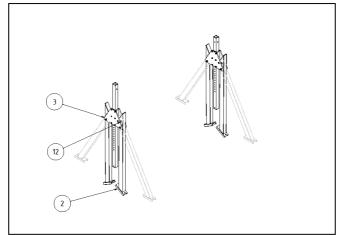
Press the push-bolt (12) provided on the stand brace (2) and open them until the push-bolts lock into place on the plastic plates (trapezium) (3).
