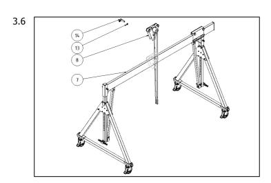
Next the trolley (8) will be placed onto the alu-beam (7). Fasten it with the plug-in bolt for the trolley (14) and secure it with a clip pin.
