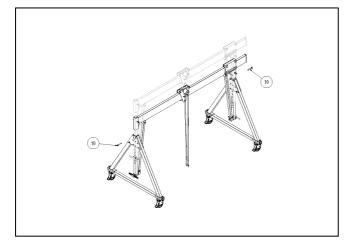
In the last step adjust the required working height by extending the beam support and fix the applicable height with a pug-in bolt (10).
