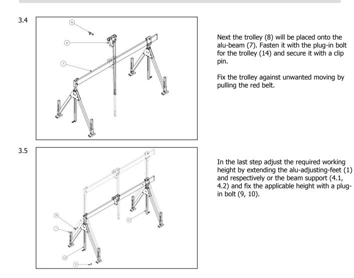
3.6 Proceed exactly in the reverse order when disassembling. Please make sure that the crane trolley is removed from the alu-beam first or fixed with the brake. The trolley will be fixed by pulling the red band and released by pulling the green band.
