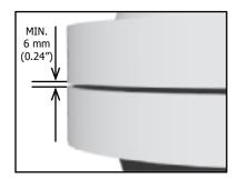
**2.** Insert the wedge into the joint until the heel of the step is in contact with the outer surface of the joint.
