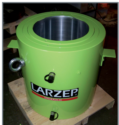
DDR200015 cylinder. 2.000 Tn capacity cylinder to place a load cell for pile testing.
